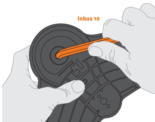
4. Turn the pressure gauge holder approximately 45° anti-clockwise until you feel resistance. Then pull out the pressure gauge holder.
