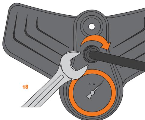
2. Pull up the pressure gauge cap.
