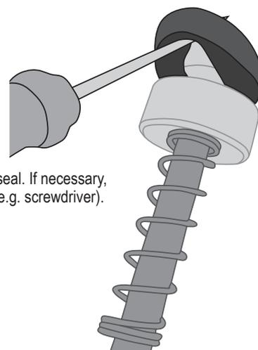
3. Place the new cup over the cylinder rod until it is positioned in the designated joint.
