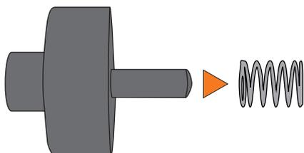
6. **ATTENTION:** Please make sure that the non-return valve system is correctly positioned in the designated fixing. Check that the spring is fitted securely!
