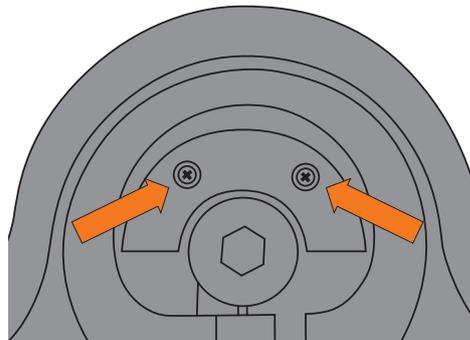
3. Lift the battery compartment cover off and replace the batteries (2 x 1.5 V AAA). It is imperative that you note the Plus and Minus symbols at the edge of the battery compartment. Insert the batteries so that the plus terminal is placed on the positive side and the minus terminal of the battery is placed on the negative terminal so that the symbols can be seen.
