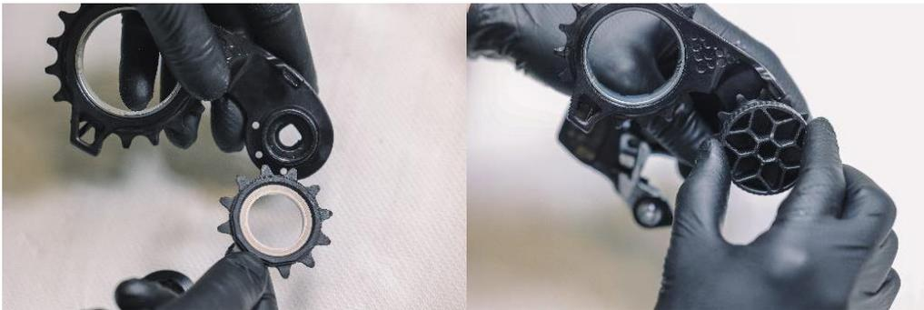
Mount the upper pulley wheel and tighten the lockring with the lockring tool to about 3-4Nm. To do that insert 8mm allen key to the lockring tool for final adjustment.
