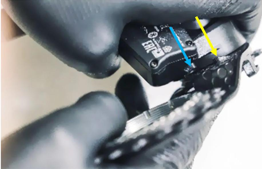
**IMPORTANT:** It is crucial to remember the position of the cage's stopper (yellow) in relation to the stopper on the derailleur body (marked with blue arrow).
